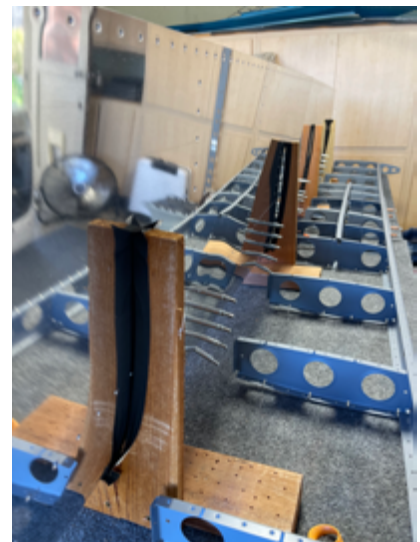
Peter Baker's RV-14A vertical stabilizer (above) and horizontal stabilizer (below) being assembled.
