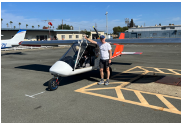
EAA 393 member Sean Cooper Kline his first young eagle in his Experimental Odyssey aircraft. His plane is powered by a 80 Hp piston engine supplemented with two turbine engines each one putting out 60 lbs of thrust.
