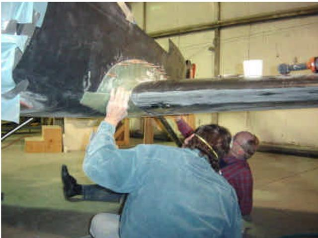
The wings are bolted onto the fuselage and the wing fairings are fitted between the fuselage and the inner edge of the wing. The fairing rib, temporarily attached to the wing, holds the fairing in the correct position on the wing, while clecos are used to attach the fairings to the fuselage. Kerry, our technician, and Harvard check the fit of the lower fairing piece.
