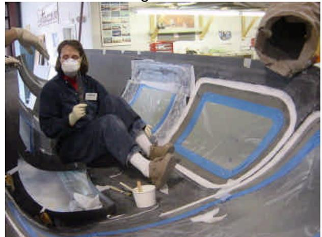
Sara is applying a mixture of epoxy and micro to fill the gaps between the windows and the inside of the fuselage skin. For the rear window, this mixture has already been covered with the carbon fiber strips and then with peel ply. The rest of the windows will be done shortly.
