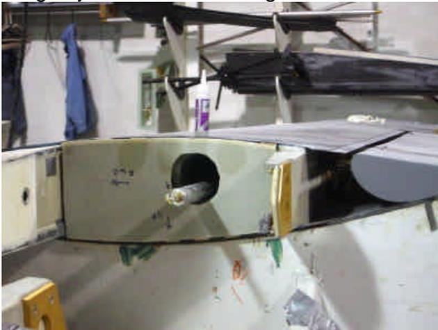
Above, Sara has cut the rib to shape and attached it to the wing with some small blocks of wood and super glue. Two more pieces, at the leading and trailing edges, are done similarly to this one between the spars.
