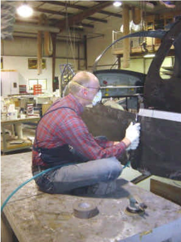
The doorframe has been fitted, marked, and then removed again, and Harvard is trimming up the fuselage to accommodate the doorframe.
